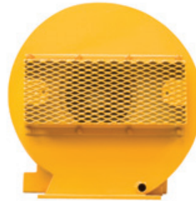
PN 260460 TDS11-HP-RH Right-Hand Top Drive Motor Blower, 5HP UL listed "XP" motor, 460V, mild steel, safety yellow
