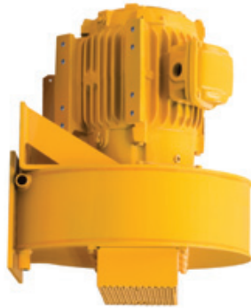
PN 260462 TDS11-HP-LH Left-Hand Top Drive Motor Blower, 5HP UL listed "XP" motor, 460V, mild steel, safety yellow
