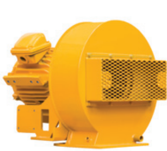
PN 260460 TDS11-HP-RH Right-Hand Top Drive Motor Blower, 5HP UL listed "XP" motor, 460V, mild steel, safety yellow
